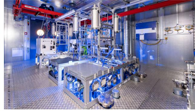
The German Aerospace Centre (DLR) is developing and testing electric propulsion systems based on hydrogen fuel cells. With the BALIS test infrastructure, a first milestone has now been reached, with two of the core components achieving an output of more than one megawatt. Together, the fuel cell system and the electric motor achieve up to 1.5 megawatts.
