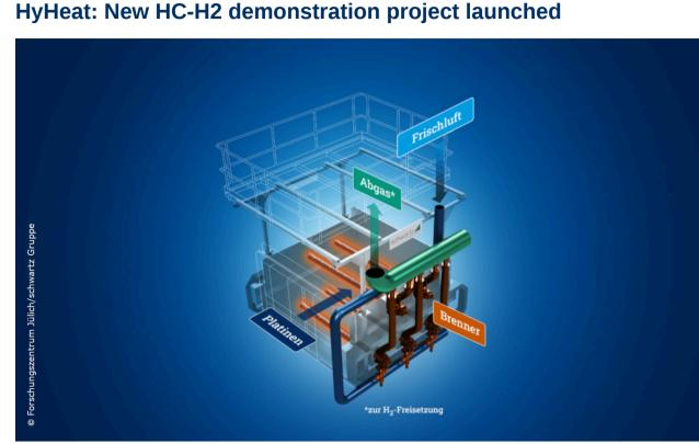
Together with new partners from the Rhineland mining region, we want to optimise industrial high-temperature processes. The Schwartz Group is the global market leader in heat treatment systems for press hardening steel, aluminium and non-ferrous metals. And that is also the focus of the recently launched HC-H2 demo project HyHeat: low-emission heat treatment of press-hardenable steel blanks.
